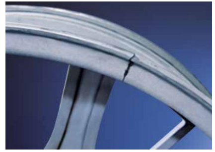
Example: Cracks - not refurbishable
