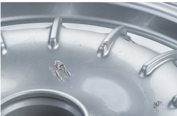
Refurbishment is NOT permitted: damage depth with 1mm in the base metal is further than 50 mm from the outer horn
