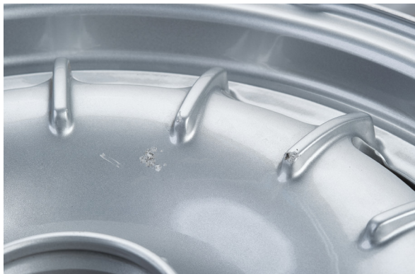
Refurbishment permitted: damages only in the paint surface
